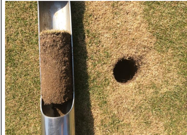
Figure 15: An inspection of the soil profile revealed hydrophobic conditions at depth with "powder dry" rootzone materials.
